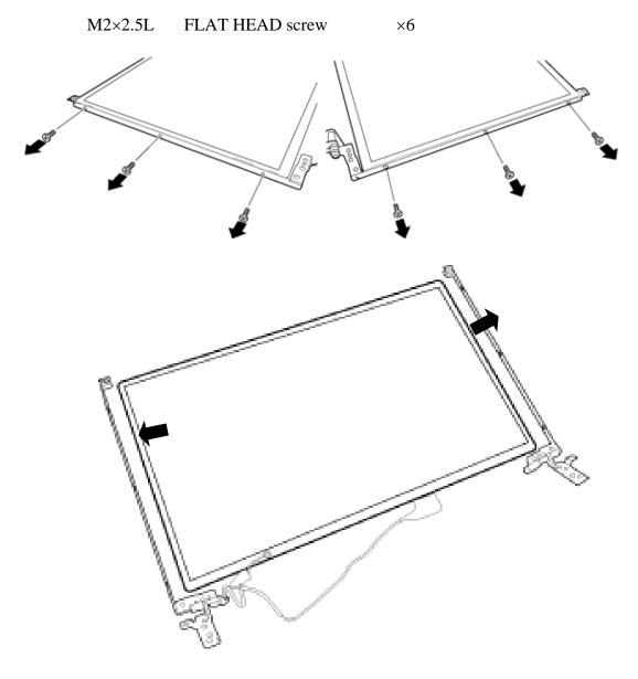
Figure 4-47 Removing the LCD supports
